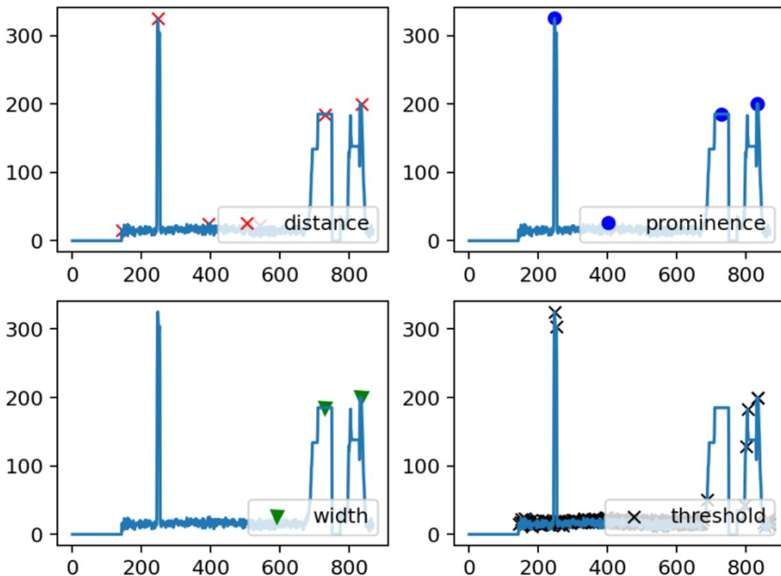
Worthy to mention that the extreme peak at the beginning is myself being close to the sensor to simulate a bird passing by or any presence of noise to the readings
