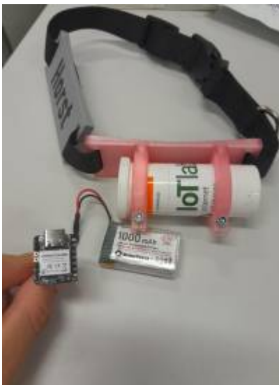
Fig. 2: Collar containing a Xiao BLE Sense module Fig. 3: Testing the prototype with an alpaca
