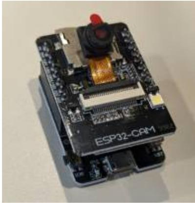
2. **Power Supply:** The ESP32-CAM requires a 5V power supply, typically provided via a USB power source.
