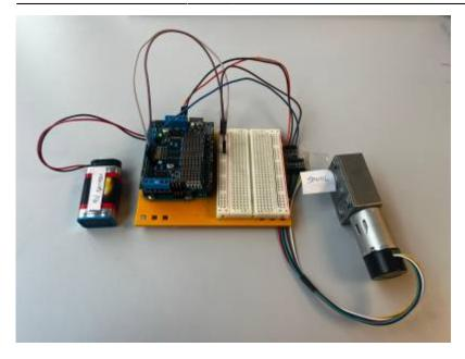
Figure 3. 12V DC worm gear motor for lowering and raising the sensor.
