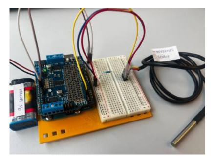
Figure 2. DS18B20 digital temperature sensor wired to digital pin D2, with a 4.7k $\Omega$  pull-up resistor between data and VCC
