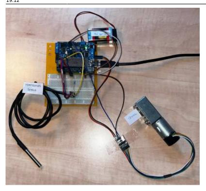
Figure 1. View of the electronics setup showing the Arduino Uno, motor shield, 9V battery and DS18B20 sensor connections
