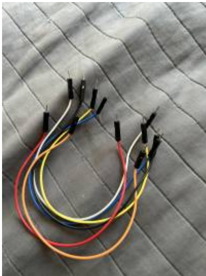
Fig 6: jumper wires (own image)
