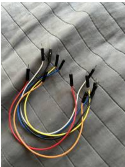
Fig 6: jumper wires (own image)
