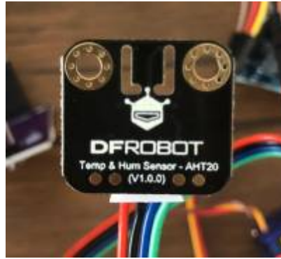
Figure 5: AHT20 Temperature and Humidity Sensor
