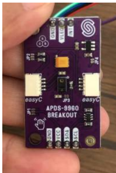
Figure 4: Gesture Sensor APDS9960 to Measure the Ambient Light Level
