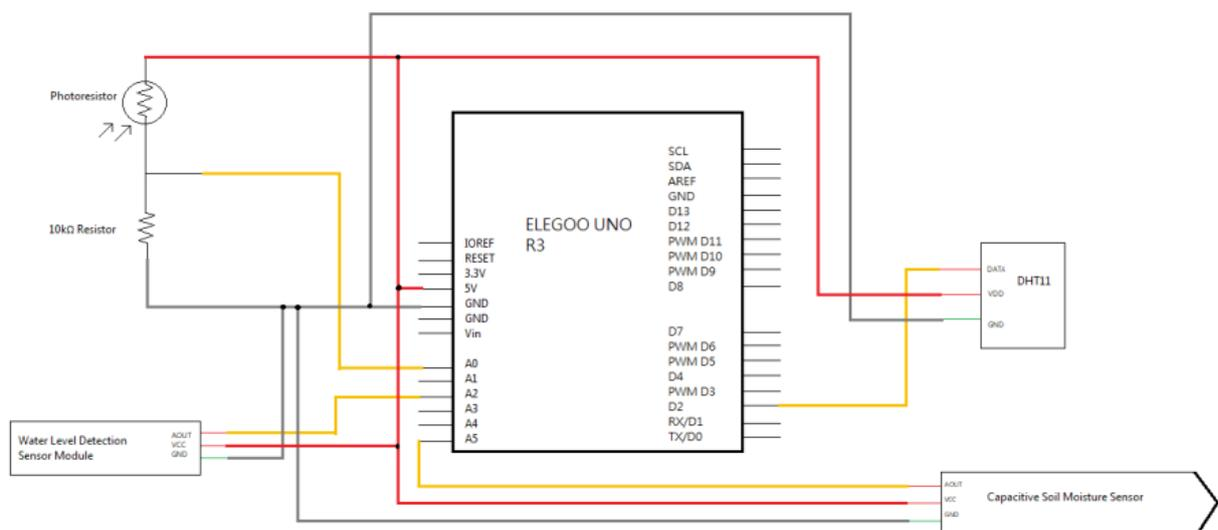
Schematic of the connection of the sensors to the Arduino board *by Veronika Skwirut*
