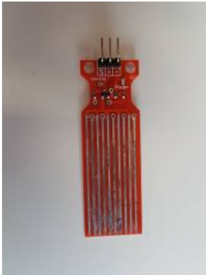
Water level detection sensor which starts to corrode, Picture by: Meinert
