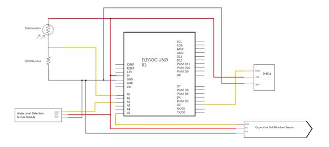
Schematic of the connection of the sensors to the Arduino board by Veronika Skwirut
