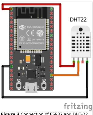
Figure 3 Connection of ESP32 and DHT-22.
