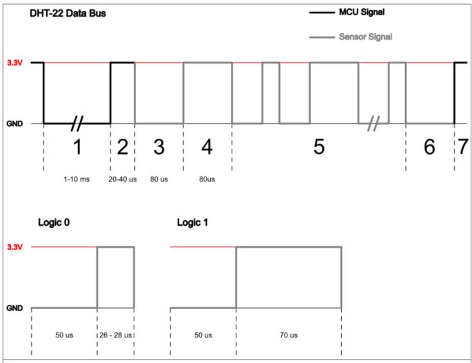
**Figure 2** Schematic of the DHT-22 communication protocol and logic '0' and logic '1'. The black line represents signals by the microcontroller, the grey line represents signals by the DHT-22.
