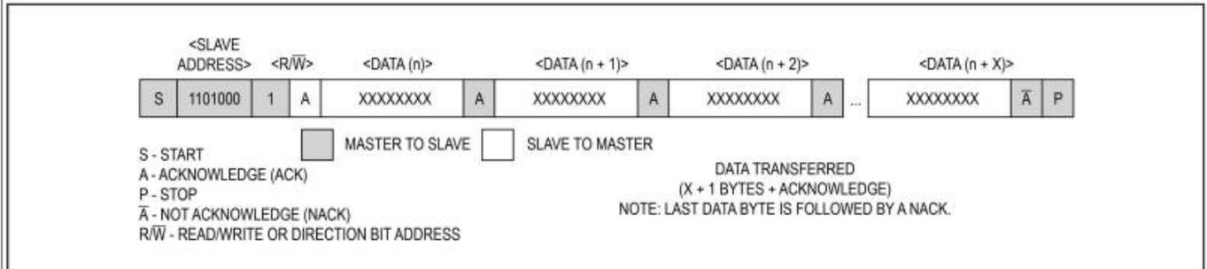
**Figure 3** Slave Transmitter Mode (Source: [DS3231 Datasheet p.16](#))
