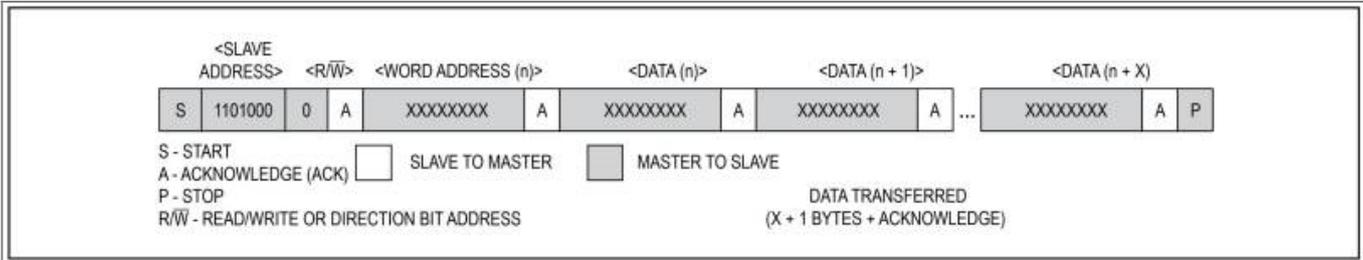
**Figure 2** Slave Receiver Mode (Source: [DS3231 Datasheet p.16](#))
