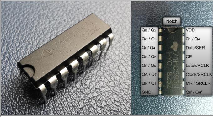
Figure 1 SN74HC595(N) Shift Register and pinout.
