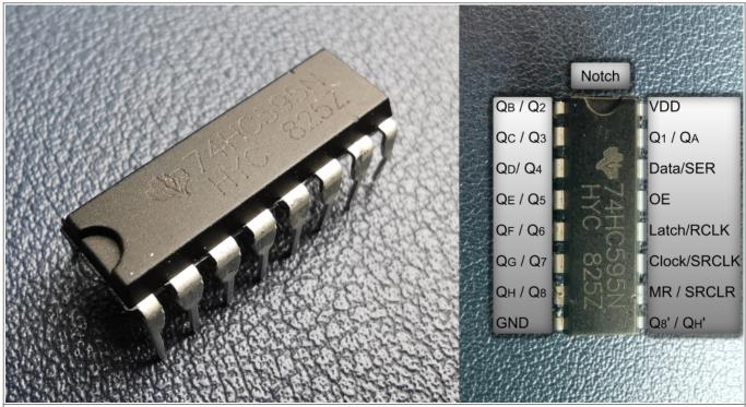
Figure 1 SN74HC595(N) Shift Register and pinout.
