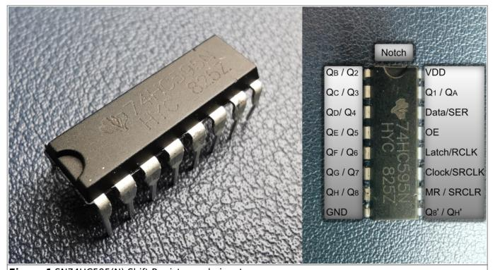
Figure 1 SN74HC595(N) Shift Register and pinout.
