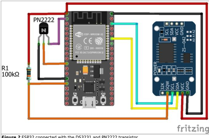
Figure 2 ESP32 connected with the DS3231 and PN2222 transistor.
