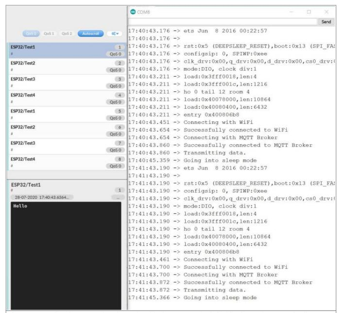
**Figure 3** Results after executing the code with the ESP32. The left side shows the MQTT.fx client receiving the 4 test messages; the result can be seen in the console at the bottom left (message posted in Test 1 was "Hello"). The right side shows the Arduino IDE's serial monitor during the process.
