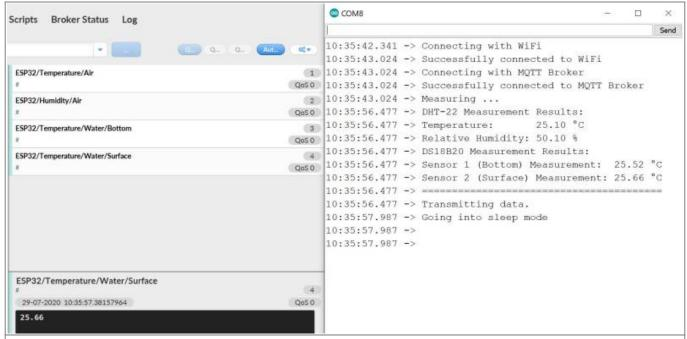
**Figure 4** Transmission of sensor data of DHT-22 and DS18B20 using MQTT. The left side shows the published measurement values in MQTT.fx; the right side shows the same results in the Arduino IDE's serial monitor.
