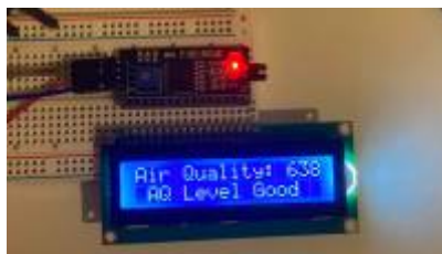
Figure 5: Liquid Crystal Display (LCD) screen (16 x 2) paired with I2C
