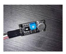
Figure 4: LM393 Microphone Sound
