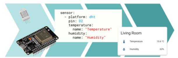
Figure: ESPHome example configuration and sensor displayed in Home Assistant, https://esphome.io/ images/hero.png
