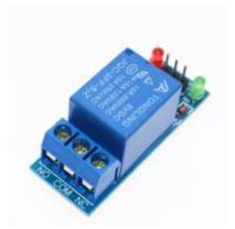
Figure: Relay module, https://www.stephenwenceslao.com/sites/default/files/1-relay-module4.jpg
