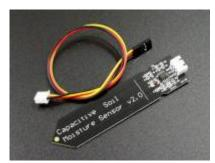
Figure: Capacitive soil moisture sensor,
