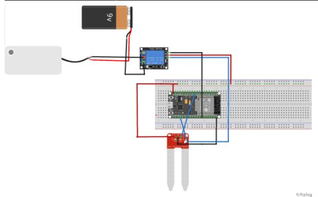
Figure: Fritzing schematic drawing of hardware setup
