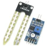
Figure: Resistive soil moisture sensor,
