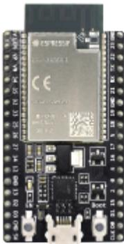
Figure: ESP32-DevKitC\_V4 with ESP32-WROVER-B,
