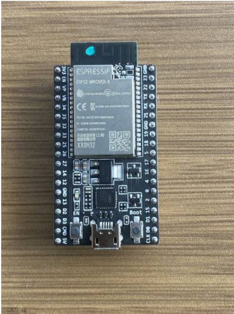
Fig.2: The ESP32 WROVER-B MODULE
