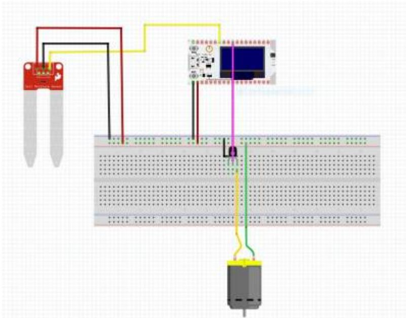
Fig4: Shows the Hardware connections,
