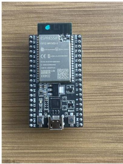
Fig.1: The ESP32 WROVER-B MODULE
