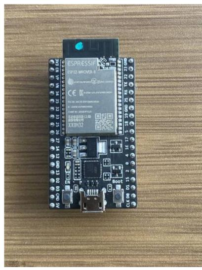
Fig.1: The ESP32 WROVER-B MODULE
