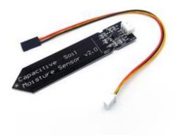
Fig.3:Capacitive soil moisture sensor.
