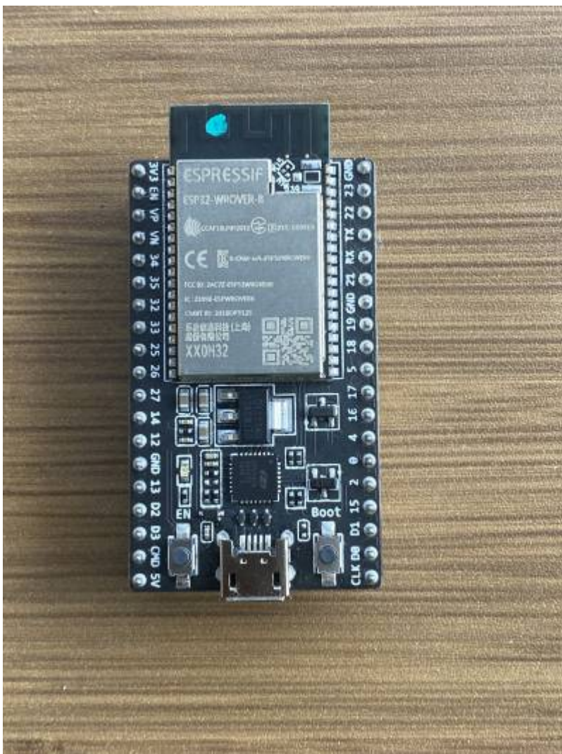
Fig.2: The ESP32 WROVER-B MODULE
