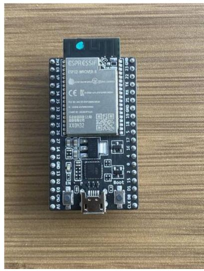
Fig.2: The ESP32 WROVER-B MODULE
