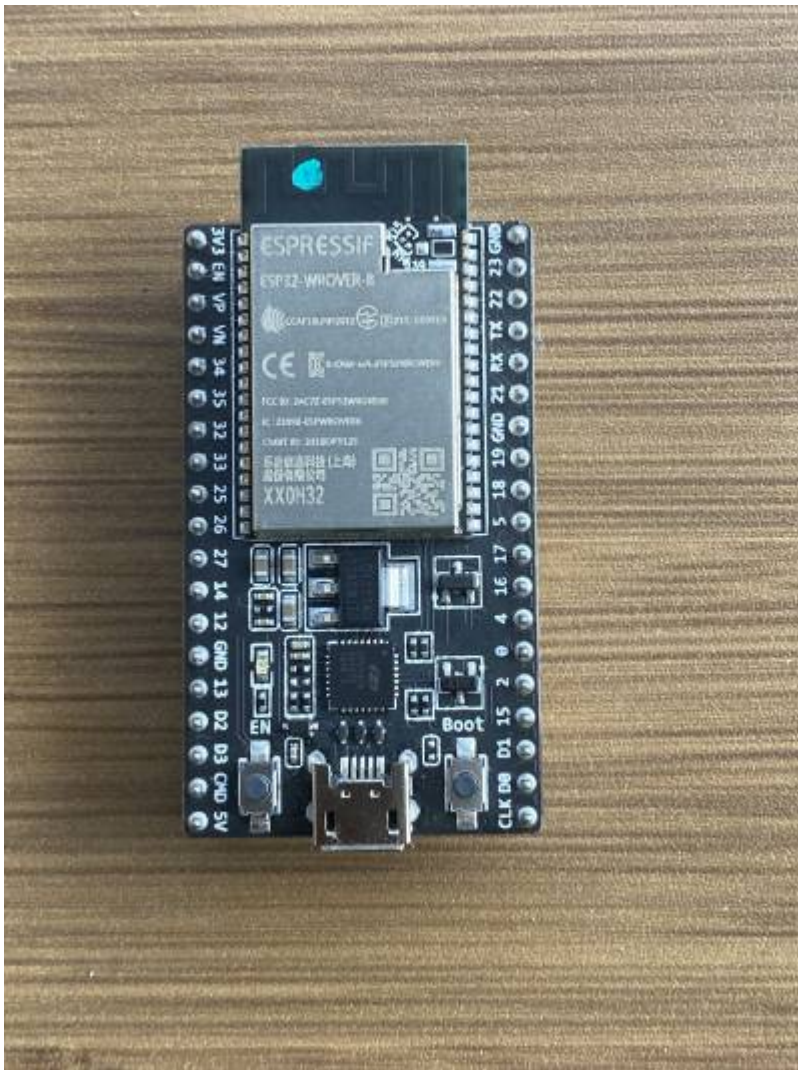
Fig.2: The ESP32 WROVER-B MODULE
