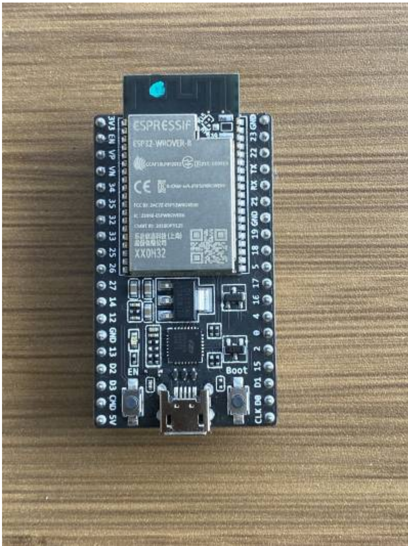
Fig.2: The ESP32 WROVER-B MODULE
