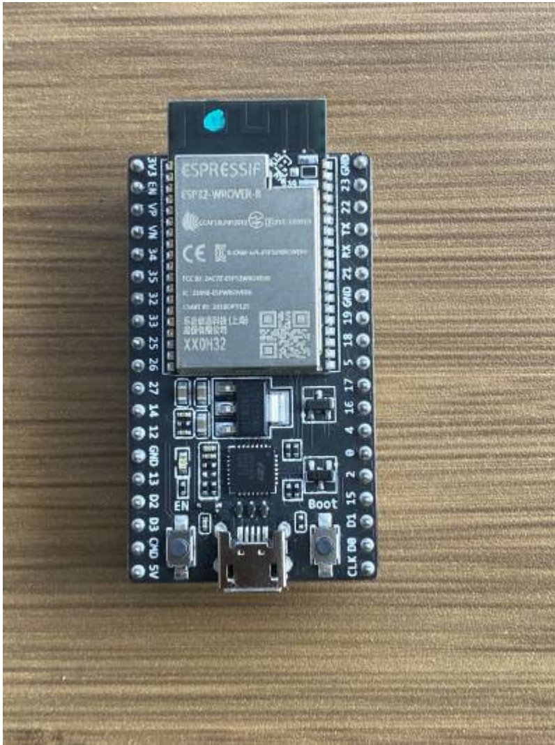
Fig.2: The ESP32 WROVER-B MODULE
