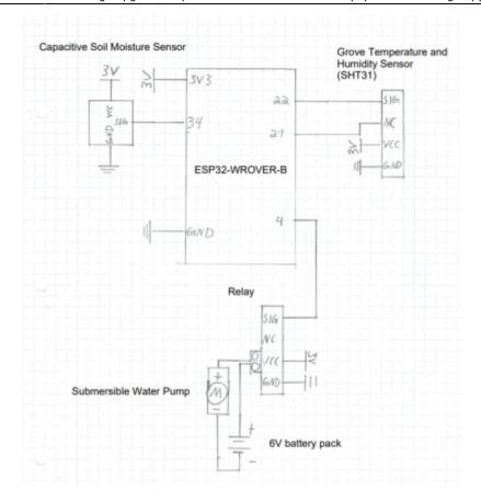
Figure 8.0 Schematics of the circuit
