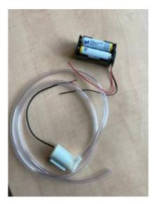
Figure 5.0 Water pump and battery pack
