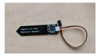
Figure 4.0 Capacitive Soil Moisture Sensor
