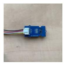
**Figure 3.0** Grove Temperature and Humidity Sensor(SHT31)
