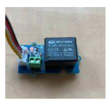
Figure 6.0 Relay Module
