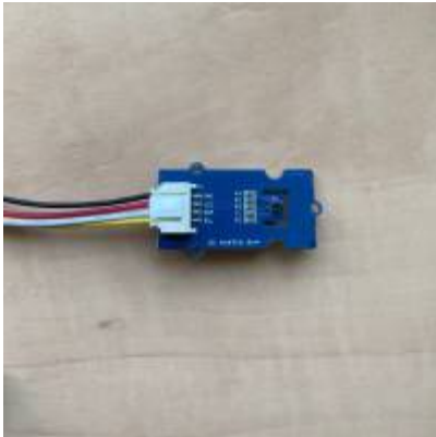
Figure 3.0 Grove Temperature and Humidity Sensor(SHT31)
