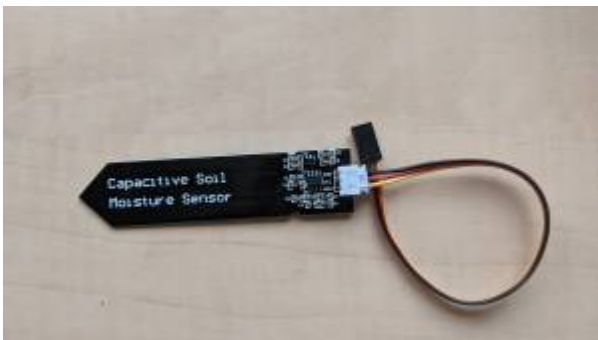
Figure 4.0 Capacitive Soil Moisture Sensor
