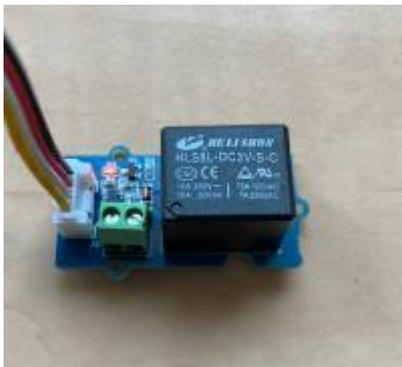
**Figure 6.0** Relay Module
