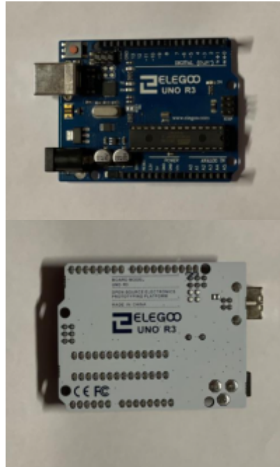
Figure 1: Arduino Uno R3 microcontroller. Source: The most complete starter kit UNO R3 Project from Rhein-Waal Hochschule.
