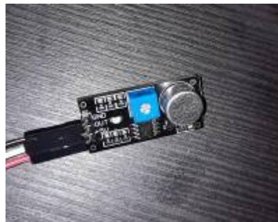
Figure 3: LM393 Microphone Sound Sensor
