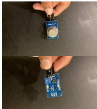
Figure 2: MQ135 Air Quality Sensor
