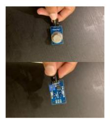
Figure 2: MQ135 Air Quality Sensor
