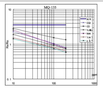
Figure 8: Calibaration graph for Mq-135
