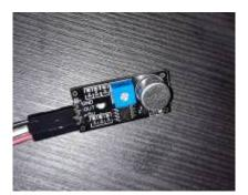
Figure 3: LM393 Microphone Sound Sensor
