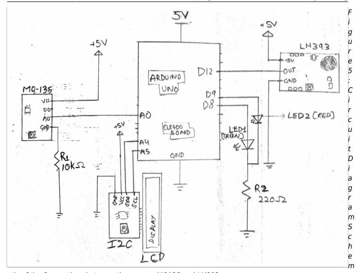
atic of the Connections between the sensors MQ135 and LM393.
