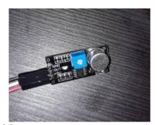
Figure 3: LM393 Microphone Sound Sensor
