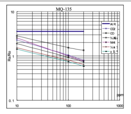
Figure 8: Calibaration graph for Mq-135
