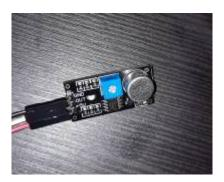
Figure 4: LM393 Microphone Sound
