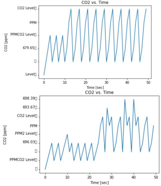
Figure 9: Screenshots of sample CO2 levels in ppm using python. Location: Meisenweg, Kamp-Lintfort. Case on the left: normal without any interference in gases detecting. Case on the right: alcohol is sprayed in the air.
