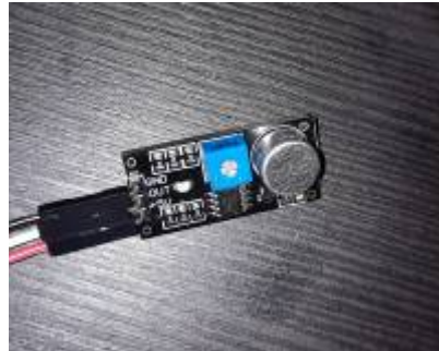
Figure 4: LM393 Microphone Sound Sensor Source: The most complete starter kit UNO R3 Project from Rhein-Waal Hochschule
