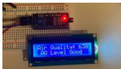
Figure 5: Liquid Crystal Display (LCD) screen (16 x 2) paired with I2C Source: The most complete starter kit UNO R3 Project from Rhein-Waal Hochschule
