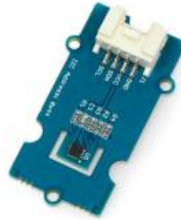
Figure 6 SHT31 Temperature and Humidity Sensor.
