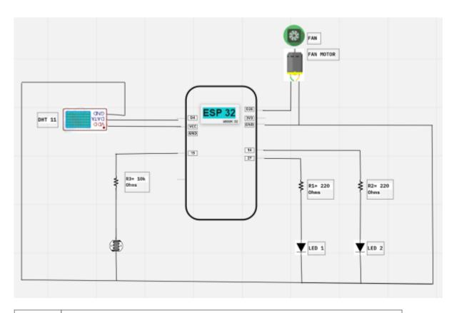
**Figure 8** Schematic Representation of the First Trial of Fan Connection to esp32.
