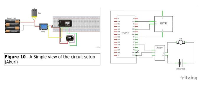
Figure 11 - Schematics of the setup (Akuri)
