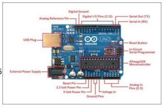
Figure 3 Arduino Uno Pin Diagram.
