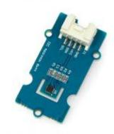
**Figure 6** SHT31 Temperature and Humidity Sensor.
