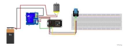
Figure 9 Change in Configuration of the fan, now moderated by a relay and 9V battery pack.
