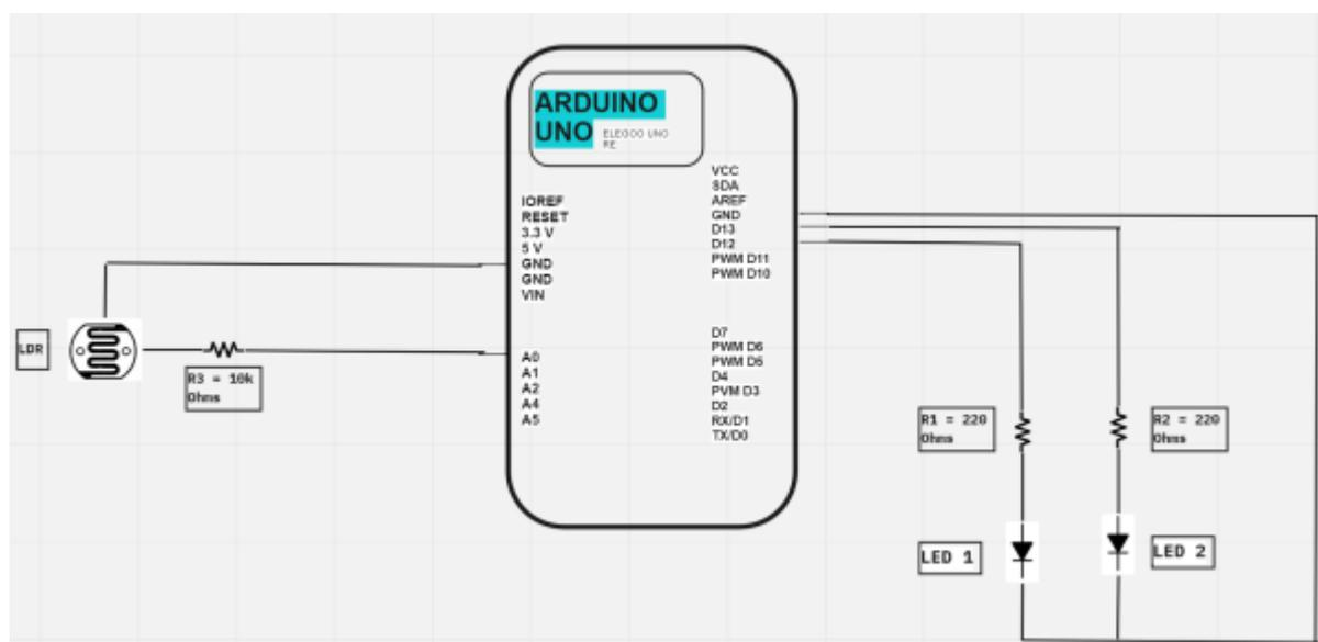
**Figure 7** LDR Setup with LEDs on Arduino UNO**4.1.2 Code**
