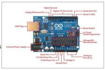
Figure 3 Arduino Uno Pin Diagram.
