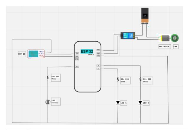
Figure 12 Complete Configuration of the Project (with DHT11 & Groove Relay), Utilized in Barbados.
