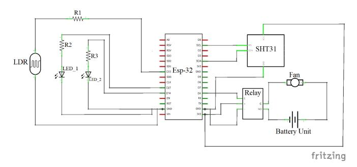
Figure 14 Complete Schematic, R1= 10K Ohms, R2 & R3 = 220Ohms, Battery Unit = 4.2 volts
