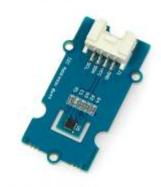
**Figure 6** SHT31 Temperature and Humidity Sensor.
