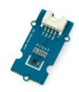
**Figure 6** SHT31 Temperature and Humidity Sensor.
