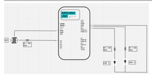
Figure 7 LDR Setup with LEDs on Arduino UNO
