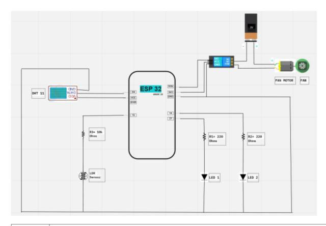
Figure 12 Complete Configuration of the Project (with DHT11 & Groove Relay), Utilized in Barbados. (Batson)
