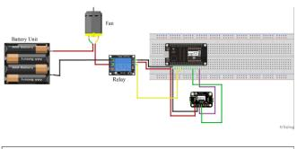
**Figure 10** - A Simple view of the circuit setup (Akuri)
