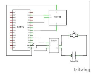
Figure 11 - Schematics of the setup (Akuri)
