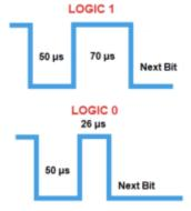
Figure # DHT22 Logic Signal formation. Source:
