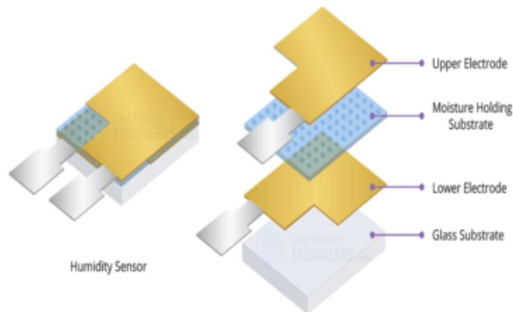
**Figure #** DHT22 sensing components. Source: <https://create.arduino.cc/projecthub/MinukaThesathYapa/dht11-dht22-sensors-temperature-using-arduino-b7a8d6//>
