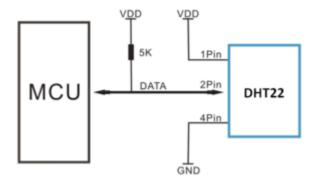
Figure # DHT22 Schematics. Source:
