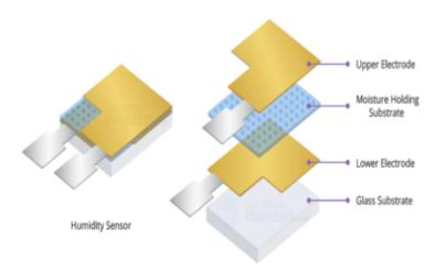
Figure # DHT22 sensing components. Source:
