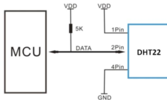
**Figure #** DHT22 Schematics. Source:
