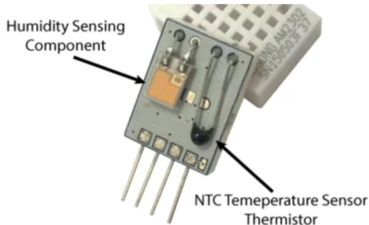
**Figure #** DHT22 Humidity sensing component. Source: <https://howtomechatronics.com>
