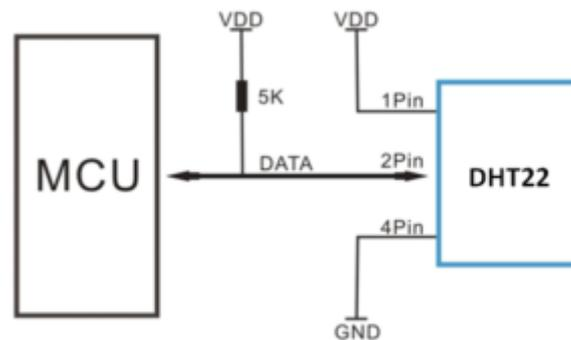
**Figure #** DHT22 Schematics. Source:
