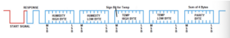
Figure # DHT22 bus transmission. Source:
