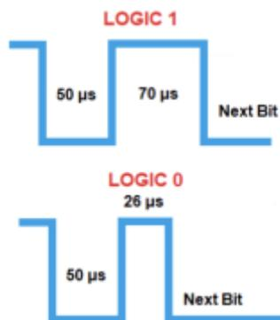
**Figure #** DHT22 Logic Signal formation. Source: <https://www.teachmicro.com/how-dht22-sensor-works///>
