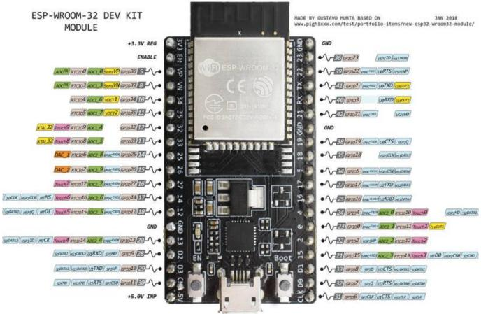
Figure 1 ESP 32 Controller. Source: https://iio.wp.com/randomnerdtutorials.com/wp-content/uploads/2018/08/ESP32-DOIT-DEVKIT-V1-Board-Pinout-36-GPIOs-updated.jpg?quality=100&strip=all&ssl=1
