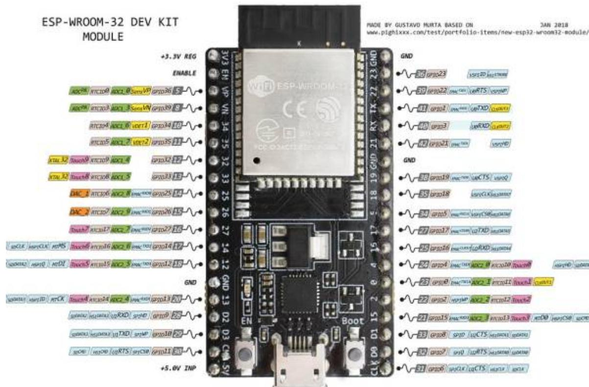
**Figure 1** ESP 32 Controller. Source:
