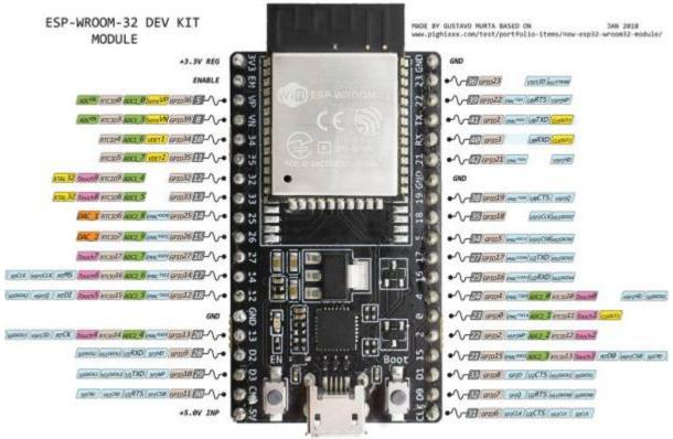
Figure 1 ESP 32 Controller. Source: https://io.wp.com/randomnerdtutorials.com/wp-content/uploads/2018/08/ESP32-DOIT-DEVKIT-V1-Board-Pinout-36-GPIOs-updated.jpg?quality=100&strip=all&ssl=1
