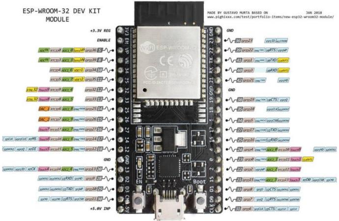
Figure 1 ESP 32 Controller. Source: https://io.wp.com/randomnerdtutorials.com/wp-content/uploads/2018/08/ESP32-DOIT-DEVKIT-V1-Board-Pinout-36-GPIOs-updated.jpg?quality=100&strip=all&ssl=1
