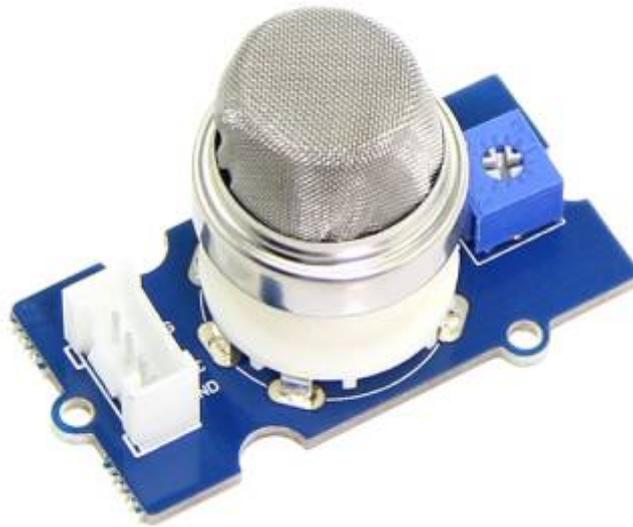
**Figure 1.** MQ2 Sensor. Source: <https://lastminuteengineers.com/mq2-gas-senser-arduino-tutorial/>
